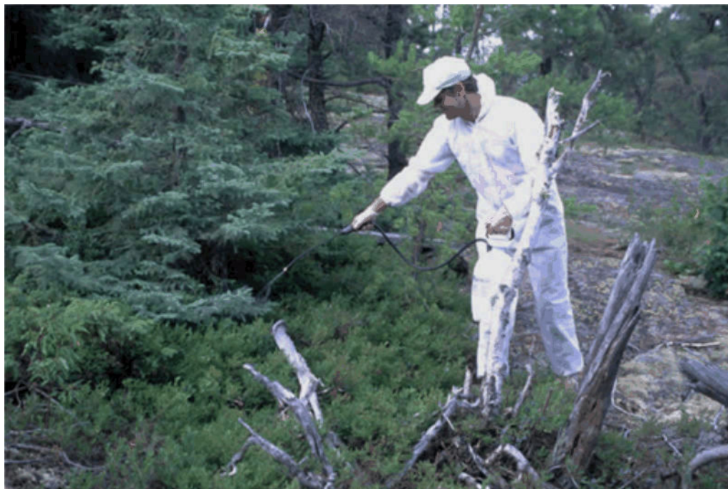
Fig. 4.80.1: ^{202}\text{Hg} was added to small watersheds to study the fate of mercury from atmospheric deposition in pristine (in its original condition) lakes as part of the METAALICUS study. (Photo Source: Toxic Substances Hydrology Program, U.S. Geological Survey) [534].
