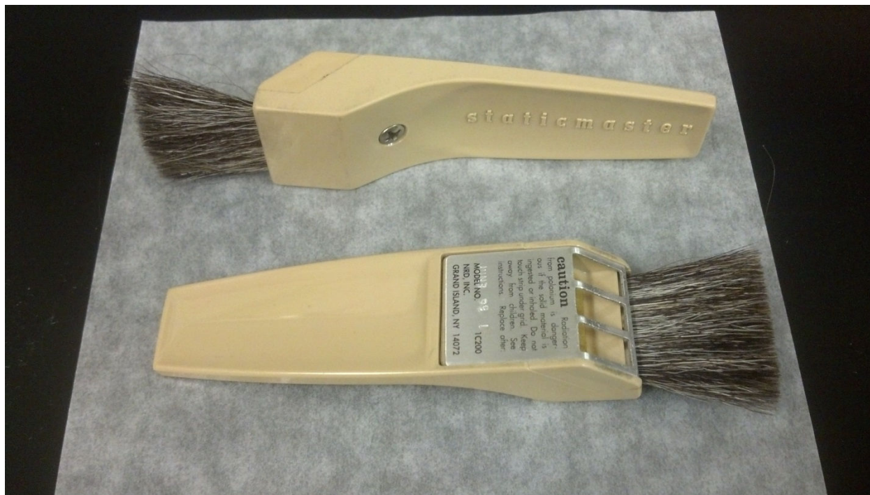
Fig. 4.84.1: Staticmaster™ Alpha Ionizing Brushes for cleaning optical surfaces and photographic films have a soft, non-abrasive brush and a ^{210}\text{Po} cartridge. (Photo Source: Reston Stable Isotope Laboratory of the U.S. Geological Survey) [561].
