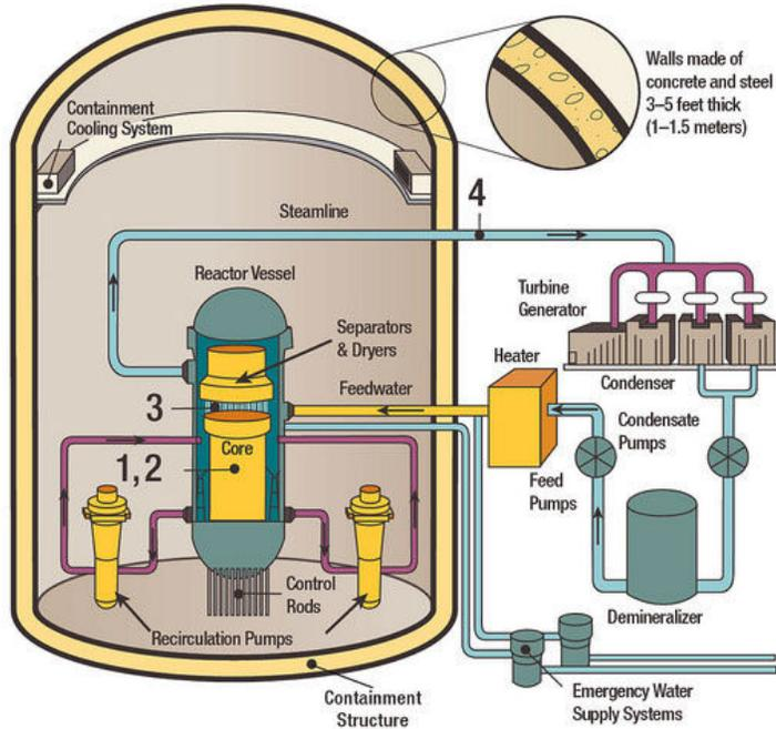
**Fig. 4.92.1:** Boiling water reactor fuel can be  $^{235}\text{U}$  enriched as uranium dioxide, which would be located in the core and is identified as “Core”. (Diagram Source: U.S. Nuclear Regulatory Commission) [599].
