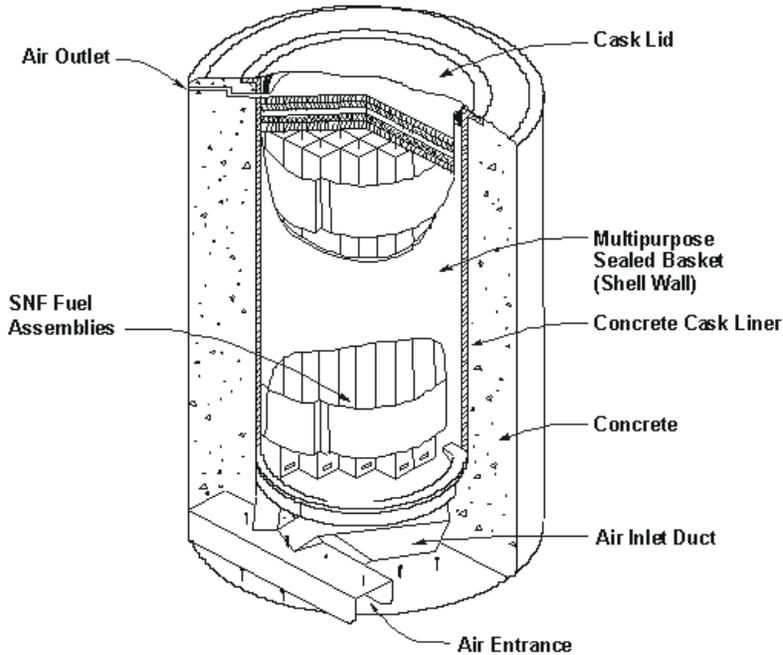
**Fig. 4.92.2:** DUCRETE cask diagram. DUCRETE is being proposed as a suitable material for the storage of radioactive waste. (Diagram Source: Argonne National Laboratory) [598].
